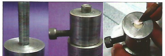
Figure 5: Specially fabricated stainless steel die (II) for vennering
