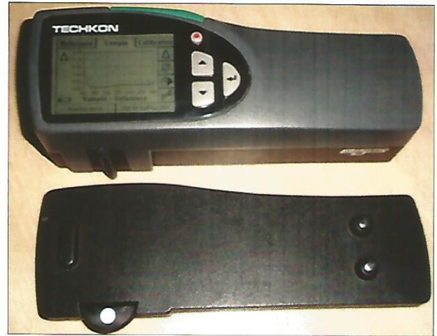
Figure 3: A portable reflectance spectrophotometer -techkon, premier colour scan
